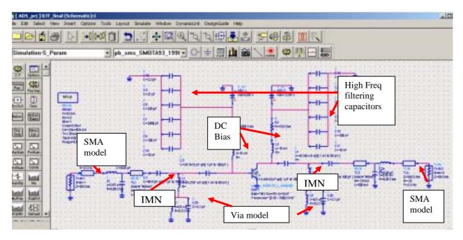
9. For the design of impedance matching network, we can use the optimization function provided in ADS to find out the appropriate capacitor and inductor values of the matching networks.
