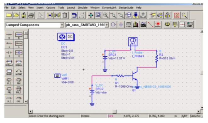
5. From the simulation result, it is known that 0.885 Vb can make the desired Ic value 8mA.
